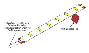
**Caution:** Do not bend, twist or crimp the lead wire at the solder connection point. This will damage the product and void the warranty.
